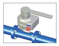
The valve is open. This can be seen by the vacant upper key slot **B** (blue) – **tOPen**. The valve cannot be operated; it is locked. The lower key **A** (red) is trapped in the key slot.
