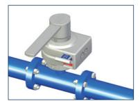
The valve is closed. The lower key  $\bf A$  (red) can be removed. Upon removal of the key the valve is locked again and can no longer be operated. The upper key  $\bf B$  (blue) remains trapped in the slot. The state of the valve (closed) is clearly visible from the vacant lower key slot.
