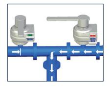
This example shows the switch over from one media (right pipe) to another (left pipe). Any mixing of both media must be avoided.
