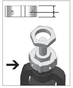
Screw the four threaded pins into the housing of the valve interlock until they are flush against the inside.
