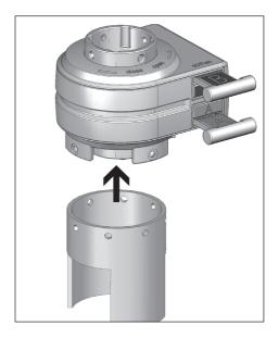
Screw two threaded pins through the holes in the torque support and tighten.
