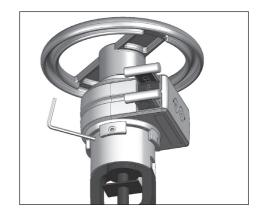
Make sure that the valve is opened all the way. Use the Tx 40 Torx key to completely remove the security screw on the right-hand side from the housing.
