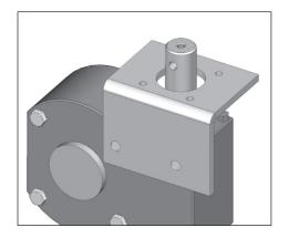
Fit the ISO shell on the gearbox spindle and tighten it using the four countersunk screws.
