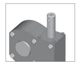
Slide the assembly bracket over the gearbox spindle in order to determine which screws of the gearbox housing need to be removed.
