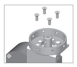
Fit the adapter on the gearbox spindle. Keep in mind that the holes in the adapter are located on the valve side (smaller edge distance).
