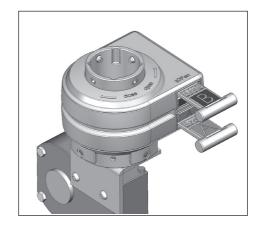
Use the four threaded pins to install the supplied handwheel. You can remove the cover of the handwheel if the valve spindle is very long.
