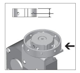
You may need to fix the adapter to the gearbox spindle in case of a shaft with transverse holes for example.
