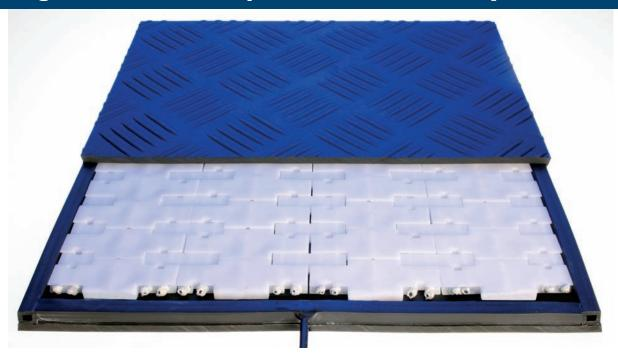
Our Safety Mats HSM® are built up of mechanically opening N/C contacts connected in series, in the form of a contact mat – similar to the unique Haake Contact Chain®.
