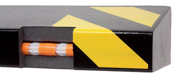
The bumper is made of soft polyurethane foam, in which the contact chains are embedded. The number and the locations of the contact chains are selected according to the size and application of the Safety Bumper.
