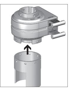
Fit the lever of the valve interlock on the shaft according to the valve position (parallel or crosswise to line). Tighten the lever with four threaded pins.
