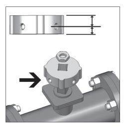
Screw the four threaded pins into the housing of the valve interlock until they are flush against the inside.
