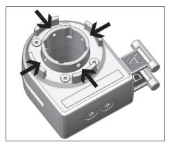
Align the valve interlock above the line so that the keys can be easily reached; four positions are possible.
